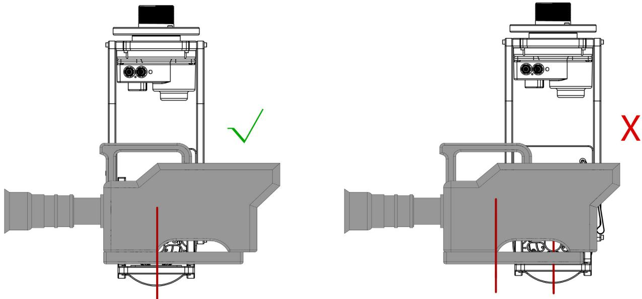
The height of the tilt motor assembly can be adjusted by loosening the 4 screws on the side plates and sliding the motor unit up or down for different camera package sizes.
