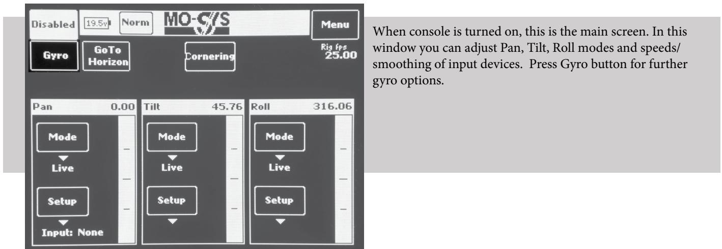
When console is turned on, this is the main screen. In this window you can adjust Pan, Tilt, Roll modes and speeds/smoothing of input devices. Press Gyro button for further gyro options.
