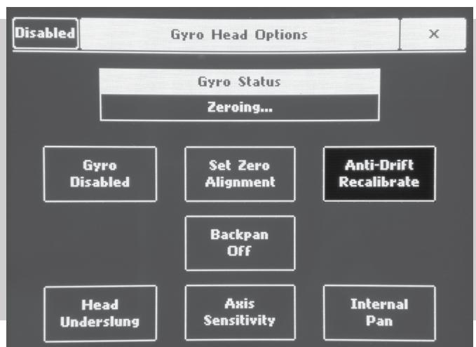
Select Backpan on or off. The Backpan feature is an option for example when using head with a crane. Pan axis of the head tracks rotation of Pan Gyro, so head keeps pointing in the same direction.
