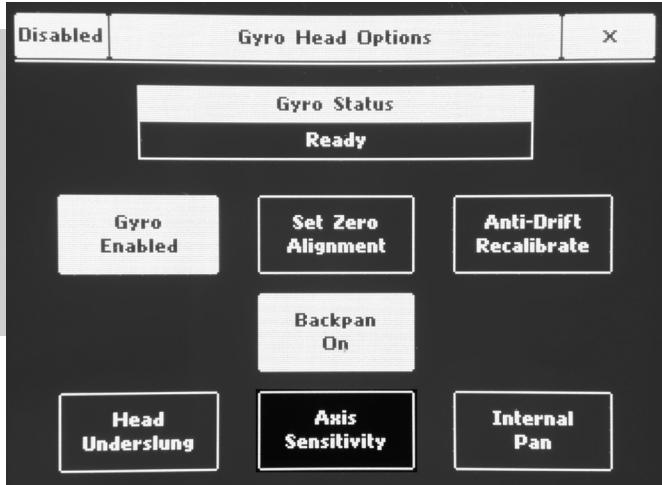
The Backpan function has adjustable sensitivity. The higher the sensitivity is set, the faster the head will track external pan motion. However, setting the sensitivity too high can lead to instability of and oscillation. So the sensitivity must be adjusted according to the solidity of the head mount. As a rule, set sensitivity to 50% initially and adjust higher until optimum performance without oscillation is observed.
